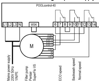
A SuperFlo VS pump can be controlled by the PC-40 unit.
