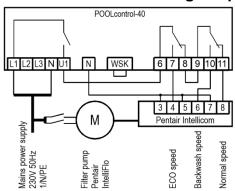
An IntelliFlo pump can be controlled by the PC-40 using the Pentair Intellicom controller.
