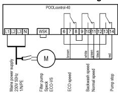
A Speck ECO-VS pump can be connected directly to the PC-40 unit. Connect the speed controller to terminals 6-14.
