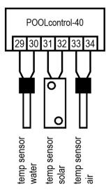
The sensors can be connected either way round (polarity not important).
