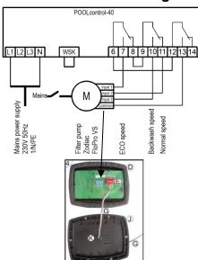
A Zodiac FloPro VS pump can be connected directly to the PC-40 unit. Connect the speed controller to terminals 6-13.
