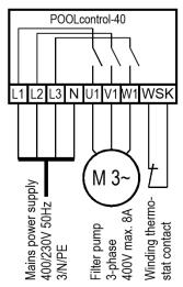
The factory-inserted link between the two WSK terminals must be removed when connecting a pump fitted with a thermal winding protection switch (winding thermostat). If the pump does not have a winding protection switch, the link must remain screwed in place. These terminals are live and carry a mains voltage!
