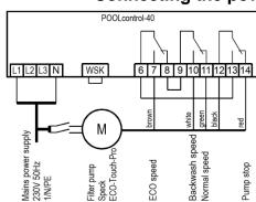
A Speck ECO-Touch-Pro pump can be connected directly to the PC-40 unit. Connect the speed controller to terminals 6-14.
