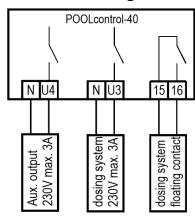
An auxiliary item of equipment running at 230V (e.g. underwater lighting) can be connected to terminal U4 and can then be timed to switch on and off by a dedicated timer in the control unit. Since this is a configurable output, it can also be used for controlling a flocculation pump.
