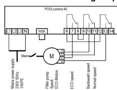
A Speck ECO-Motion pump can be connected directly to the PC-40 unit. Connect the speed controller to terminals 6-13.
